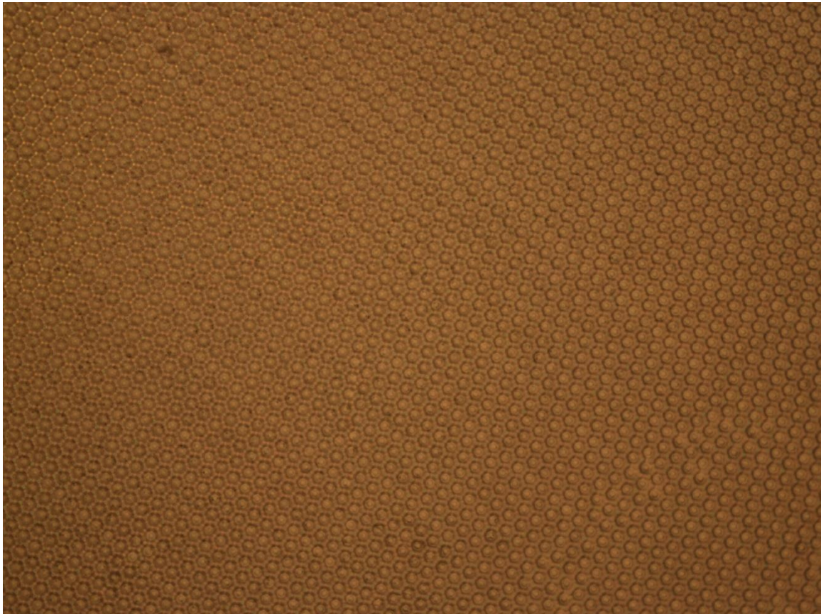
Figure 2: hexagonal pattern obtained by photolithography
