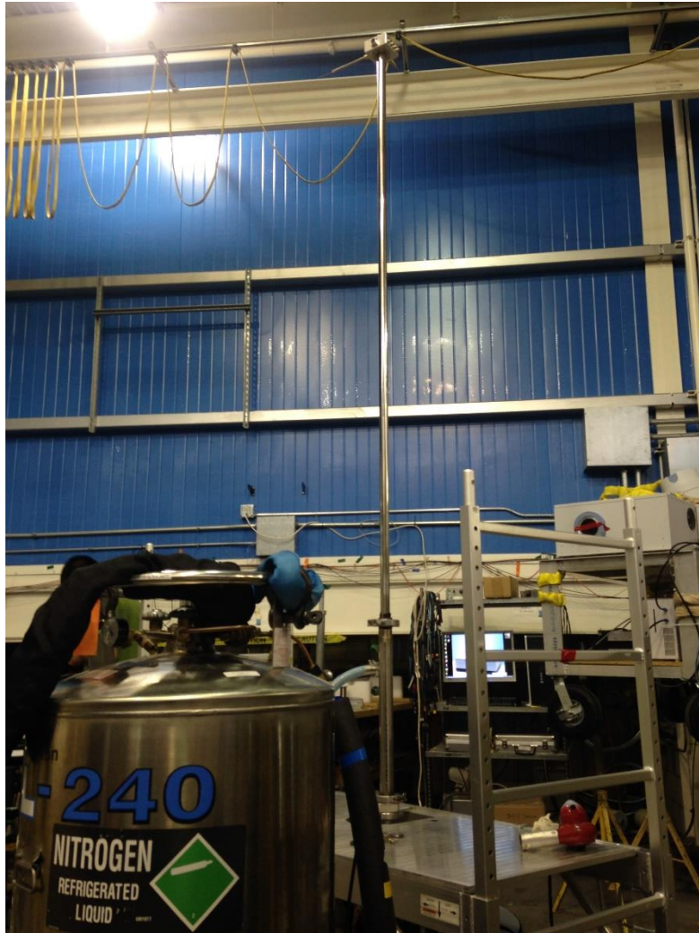
Figure 3: sliding probe down into the fridge
